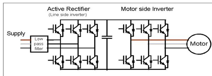
**Figure 10 Basic active rectifier voltage source inverter**
