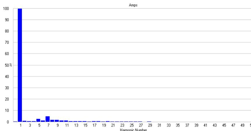
**Figure 11 Typical measured current harmonic spectrum for active rectifier drive (THDi = 3.5%)**
