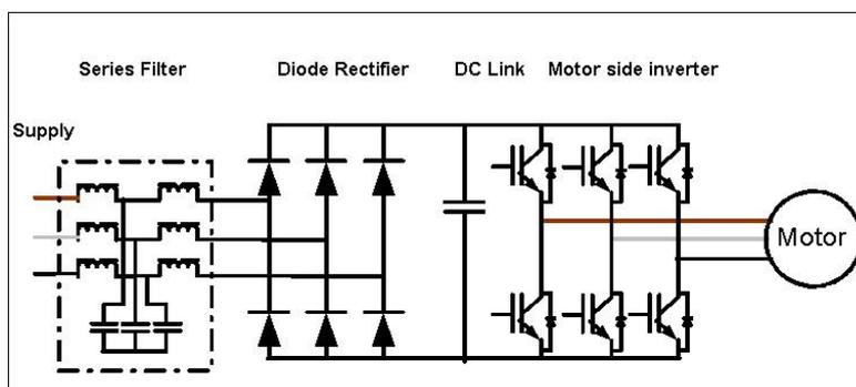
**Figure 13 Voltage source inverter with series filter**
