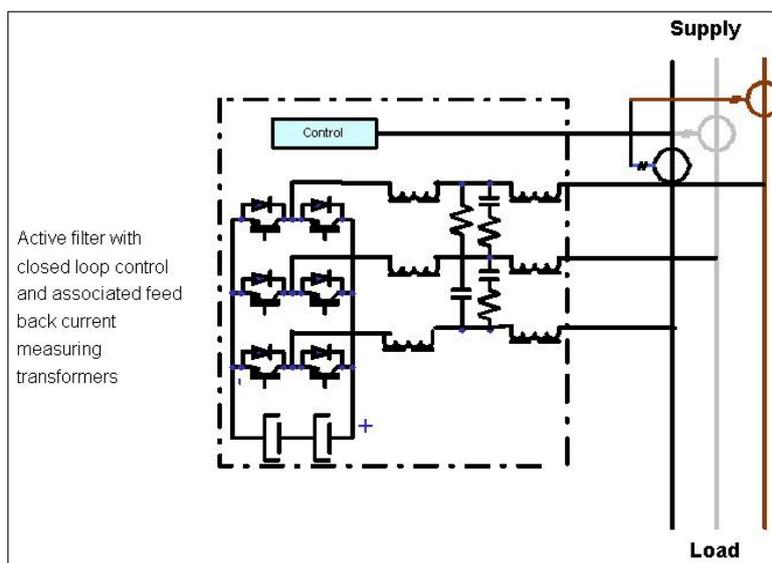
**Figure 14 Typical closed loop active filter**
