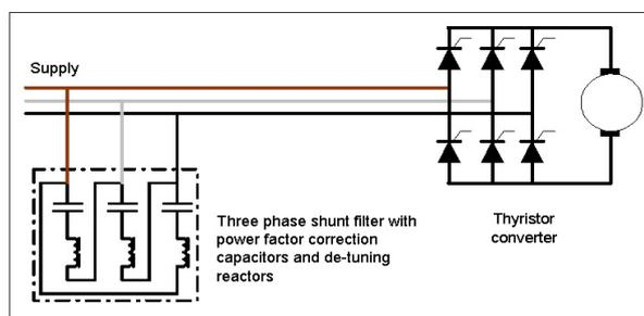
**Figure 12 d.c. converter with shunt filter**
