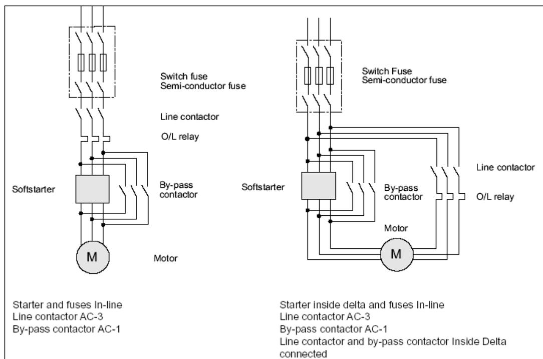
**Figure 15 - Typical soft starter connections**
