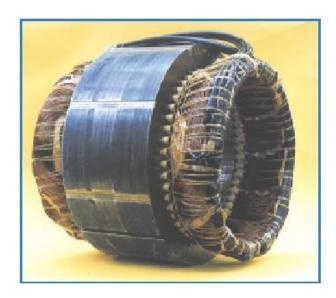
Figure 18 Completed random winding
