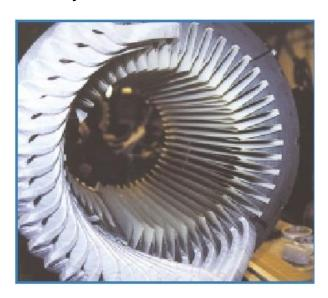
Figure 17 Partially wound stator core with form winding
