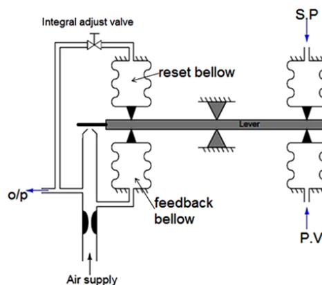
Fig 3 – Pneumatic PI Controller Fundamentals <sup>(4)</sup>
