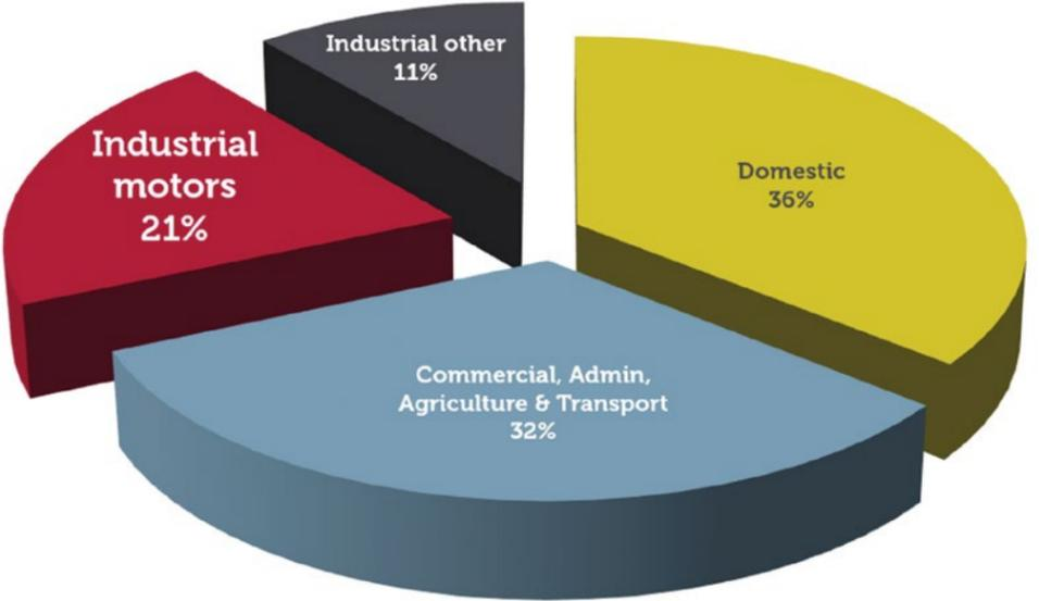
Some 21 percent of UK electricity consumption is by industrial electric motor driven systems
