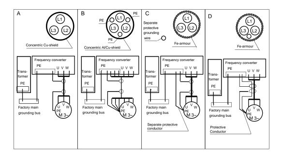
Figure 4 Typical Converter/Motor Cables
