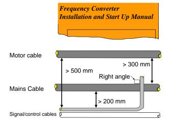
Figure 10 Recommended Segregation between cables
