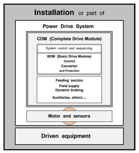
Figure 1 - The Power Drive System
