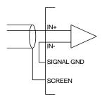
Figure 9 - Incorrect control cable connection
