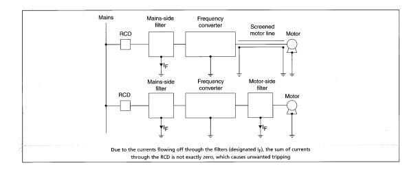
Figure 11 Interference paths for RCD operation
