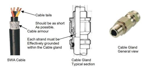
Figure 6 - Typical Cable and Gland
