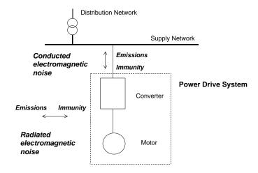
Figure 13 EMC aspects of a power drive system
