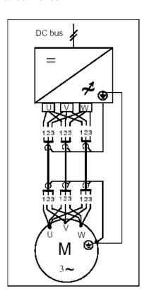
Figure 5 - High Current Installation
