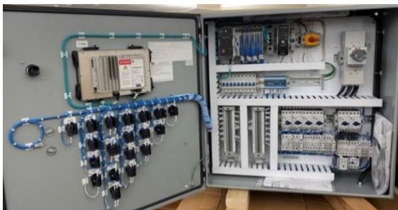
**Figure 8 – Wiring of a conventional panel**
