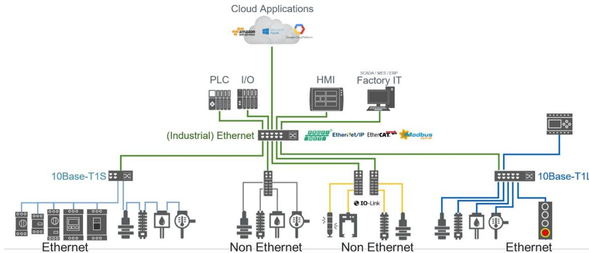
**Figure 11 – Draft of an IP everywhere network architecture.**
