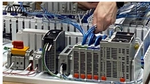
**Figure 9 – Conventional control panel wiring**
