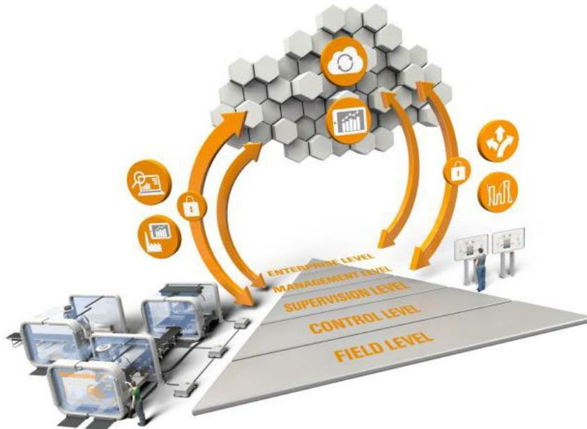
**Figure 2 – IIoT architecture**
