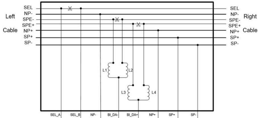
**Figure 25 – Plug connector P1 circuit.**
