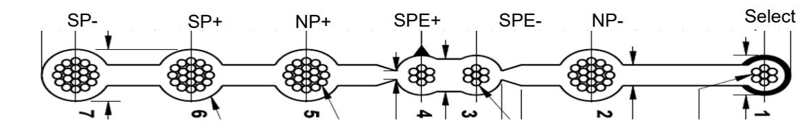
NP and SP lines are rated at four Amps. The unique cable design, featuring an asymmetrical arrangement of conductors, prevents incorrect connector orientation.
