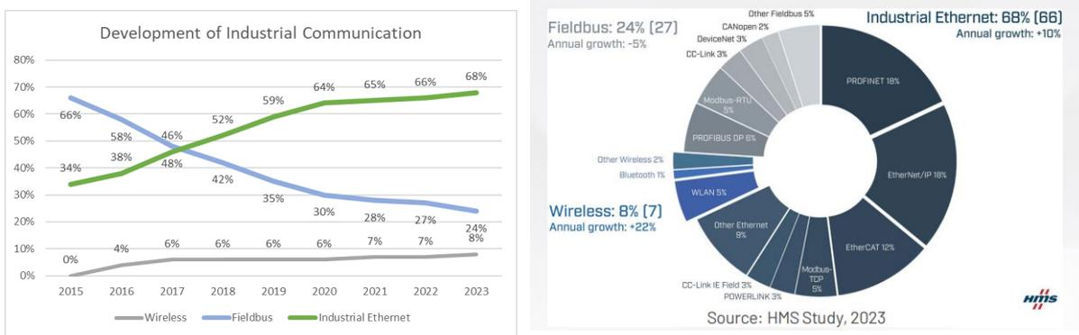
Figure 3 – Fieldbus transition to Ethernet
