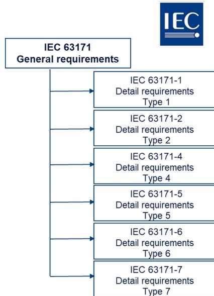
**Figure 14 – The IEC 63171 series of connector standards.**
