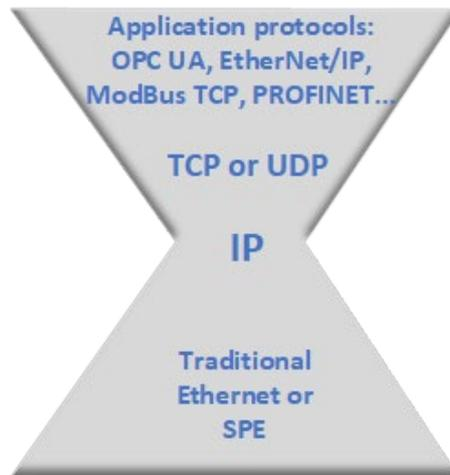
**Figure 10 – The pivotal role of the IP layer.**
