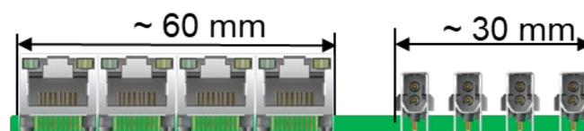
**Figure 20 – Space comparison of an IEC 63171-2 connector with RJ45.**
