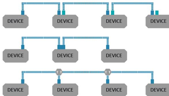
Figure 22 – Examples of multidrop implementations
