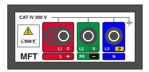
This typical multifunction tester terminal panel is rated for CAT IV 300 V measurement connection. Measurement connection to CAT IV, CAT III or CAT II circuits may be made provided voltage does not exceed 300 V with respect to earth. Measurement connection not exceeding 550 V between phases may be made provided no voltage exceeds 300 V with respect to earth.
