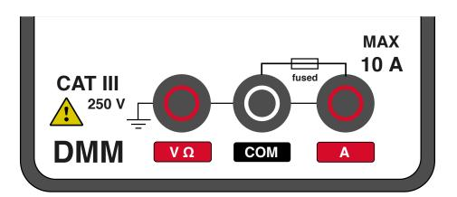
This multimeter is rated for mains measurement connection up to CAT III 250 V with respect to earth.
