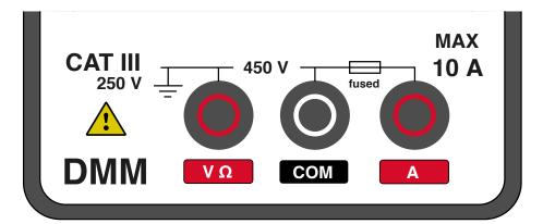
This multimeter is rated for mains measurement connection up to CAT III 250 V with respect to earth and 450 V between terminals.
