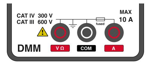
This multimeter is dual rated for mains measurement connection up to CAT IV 300 V with respect to earth, and to CAT III 600 V with respect to earth.
