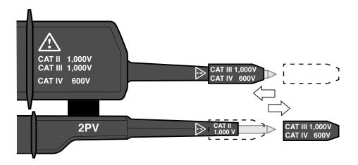
This two-pole voltage detector is rated for measurement connection to CAT II 1,000 V, or CAT III 1,000 V and CAT IV 600 V.
