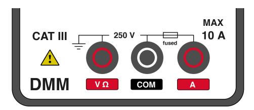
This multimeter is rated for mains measurement connection up to CAT III 250 V with respect to earth and 250 V between terminals.
