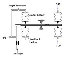
Fig 3 – Pneumatic PI Controller Fundamentals <sup>(4)</sup>
