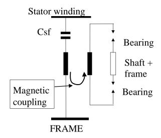
Figure 17 - Equivalent circuit for circulating current
