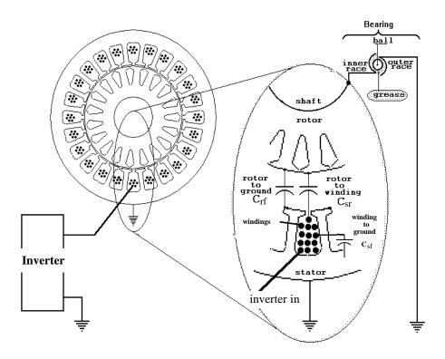
Figure 9 - Capacitances of motor winding
