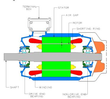
Figure 1 shows a longitudinal view of an induction motor with its constituent parts.
