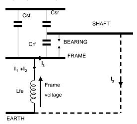
Figure 14 - Shaft grounding current equivalent circuit
