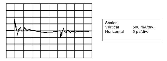
Figure 10 - Typical waveform of motor frame earth current
