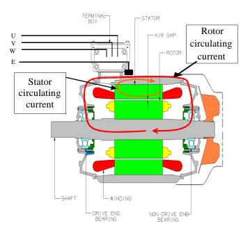
Figure 16 - Induction of rotor circulating current
