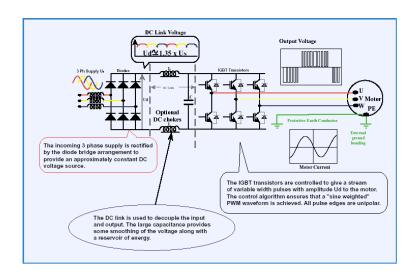
Figure 5 - Basic elements of voltage source inverter
