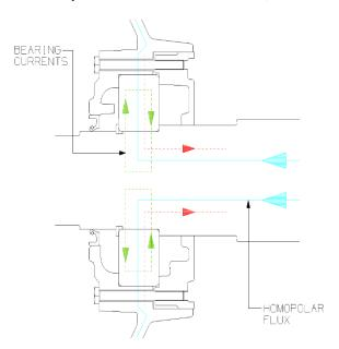
Figure 4 - Currents adding in a bearing
