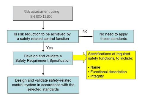
Figure 5 – Application of EN 62061 and EN ISO 13849-1
