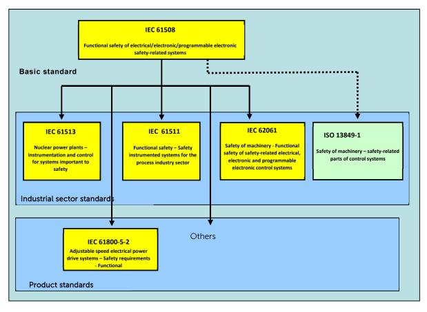
Figure 7 - The IEC 61508 family of functional safety standards (EN versions are also described in the text)
