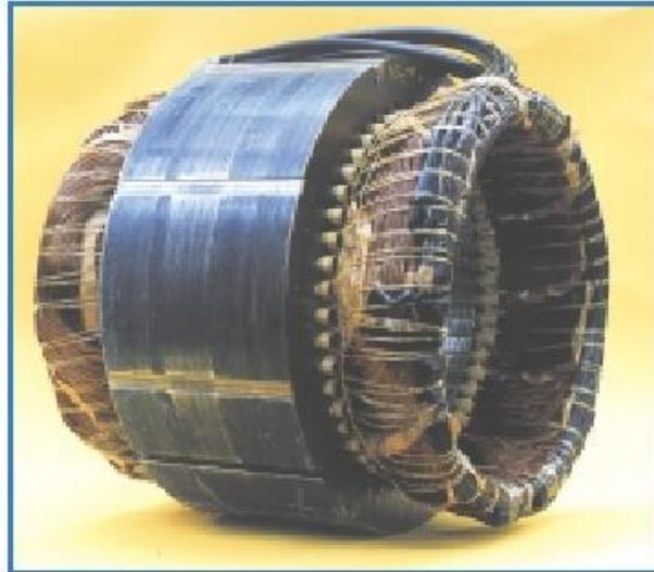
**Figure 18 Completed random winding**
